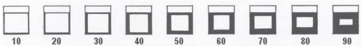
b) Guide for estimating fracture appearance
